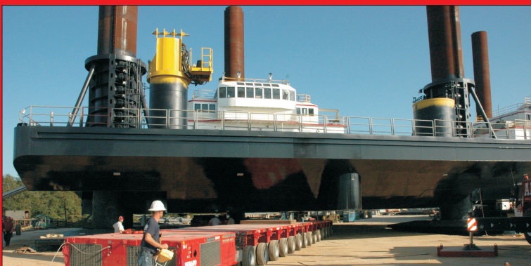
Brad Courville setting the SPMT's under the massive load.
